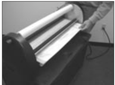
Photo 10-4: Threading board and film web exiting pull rollers.
