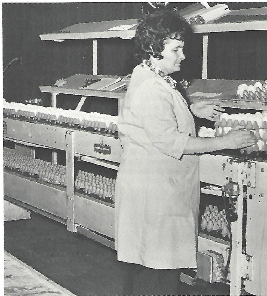
At the processing plant, flats of eggs are placed on the conveyor of a Diamond PA-120 automatic loader. The flats are returned automatically to the stacker. Later the flats are run through a flats washer.
