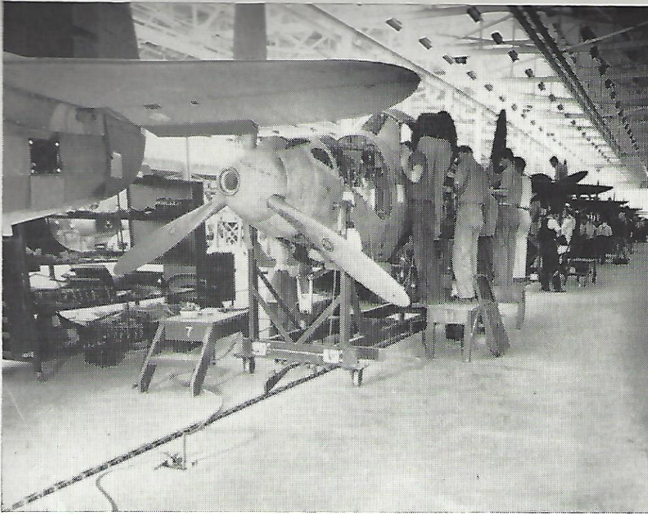
Nearing the end of the final assembly line. Notice conveyor track set in floor and device which moves the dolly slowly along as work proceeds on the ship.
