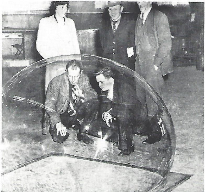
To shield the pilot and passenger from the elements, Young (kneeling at left) invented this protective bubble enclosure for Ship 3.
