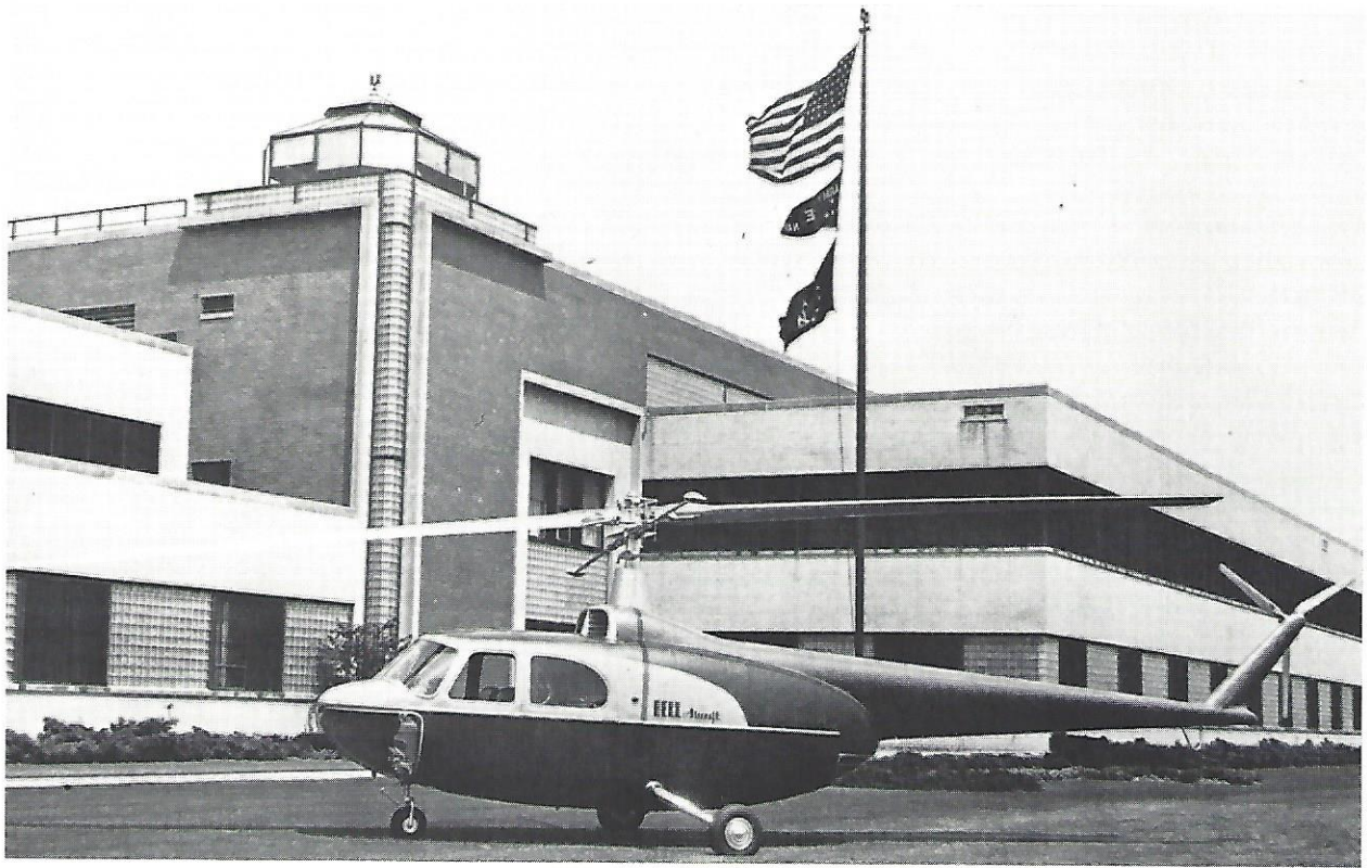
Bell Aircraft had great expectations for the streamlined five-place Model 42 that was designed on the basis of a marketing survey.
