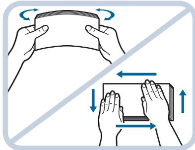
1. Place the envelopes on a clean, level surface, and press all the way around the envelopes by hand, in the direction of the arrows, to remove any curls.
