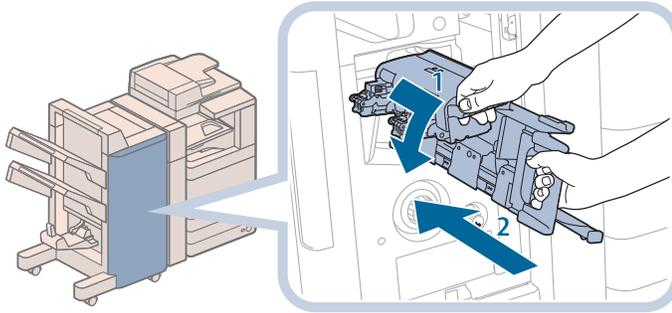
1. Pull the stapler unit of the saddle sticher unit towards you, and then push it down into its original position.
