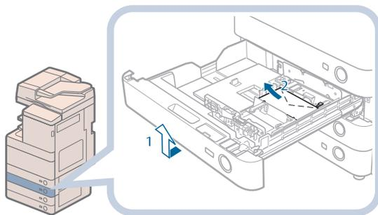
1. Pull and lift the paper drawer out of the machine by holding its left and right sides with both hands.
