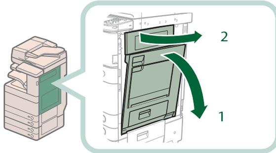
1. Grip the handle, and open the lower right cover of the machine.
