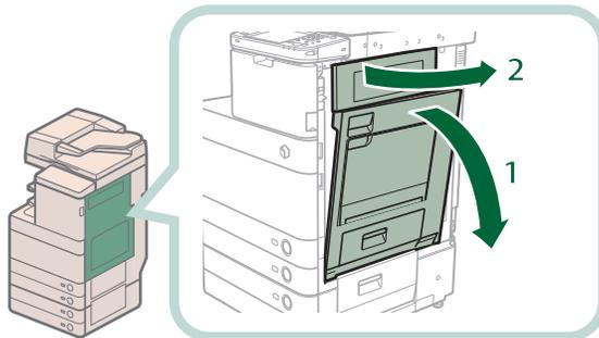
1. Grip the handle, and open the lower right cover of the machine.
