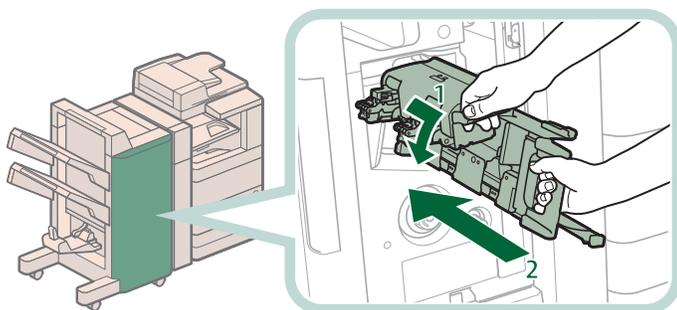
1. Pull the stapler unit towards you, and then push it down into its original position.
