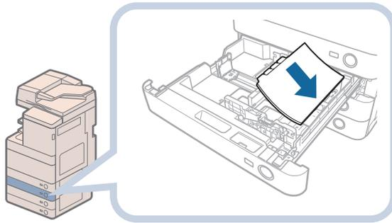
Load the tab paper face up with the tabs to the left side, as shown in the illustration below.
