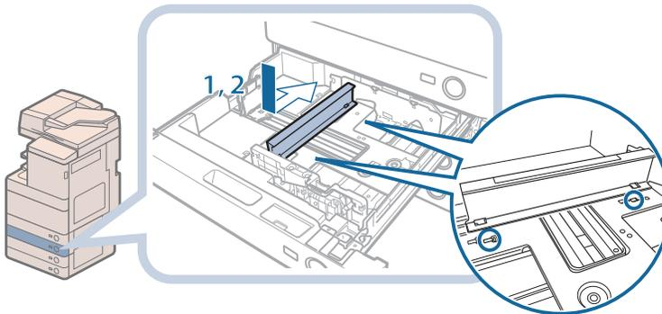
1. Place the Tab Feeding Attachment Kit-B1 into the holes of the paper drawer.
