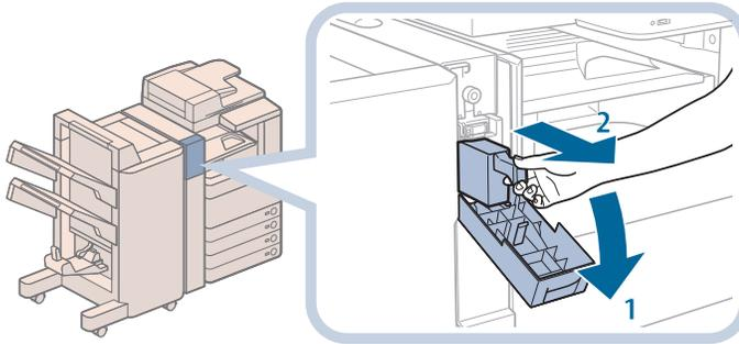
1. Open the front cover of the puncher.
