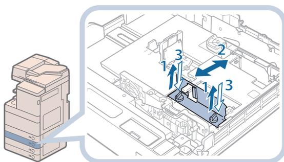
1. Loosen the two screws fixing the front width guide of the envelope feeder attachment.
