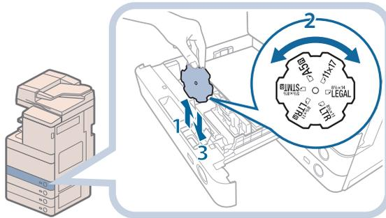
1. Open the inside cover of the paper drawer, and lift up the plate.
