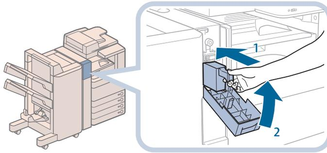
1. Push the punch waste tray back into its original position.
