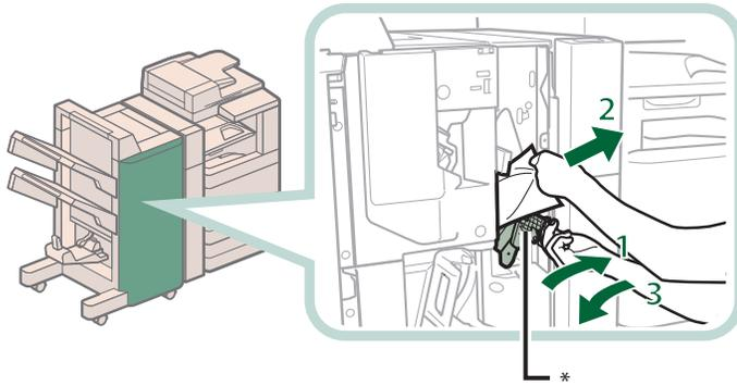
1. Turn the lever on the lower delivery guide to the right until it stops, and then tilt the lower delivery guide to the right.
