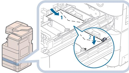
1. Load 10 envelopes at a time with the side you want to print on facing up. While loading the envelopes, press down on the left side of the receptacle to lock them into place.
