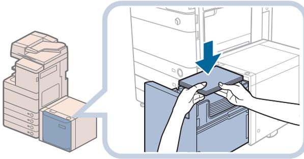
1. Load the paper stack against the back left guide of the paper deck unit.
