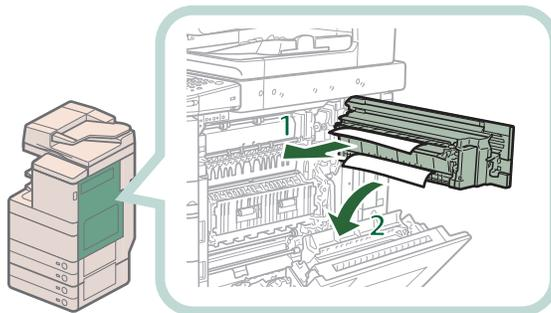
1. Remove any jammed paper in the upper part of the duplexing unit.
