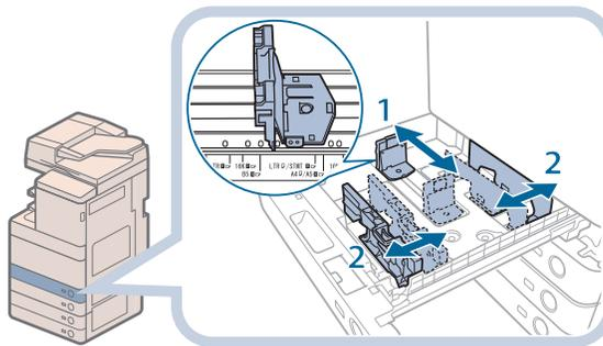
1. Slide the left guide while squeezing it on the top to align it with the mark for the desired paper size.
