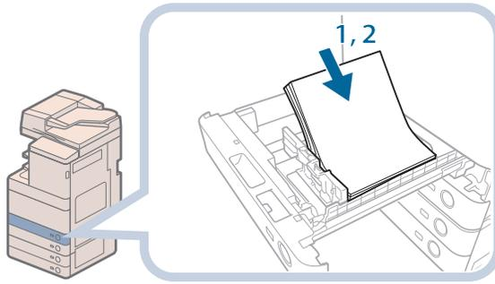
1. Make sure that the paper size setting of the paper drawer matches the size of the paper to load in the paper drawer.
