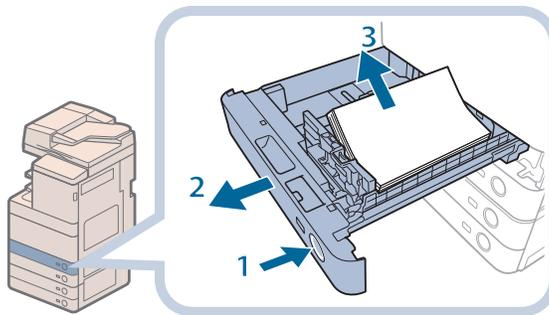
1. Press the open button on the paper drawer for which you want to adjust the paper size.
