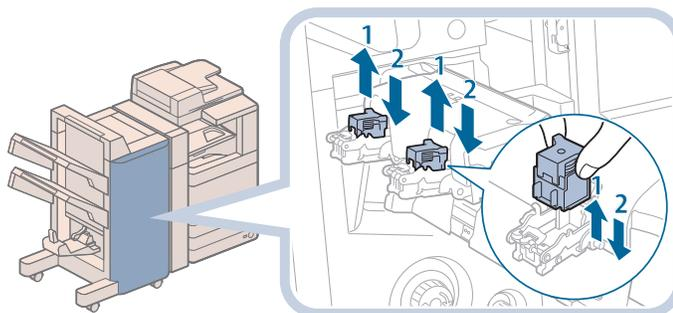
1. Pull out the empty staple case, holding it by its left and right sides.
