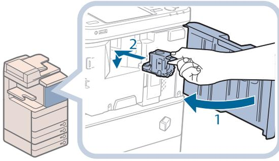
1. Gently push the staple case back into the finisher and push down firmly until it is securely in place.
