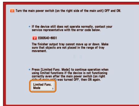
If [Limited Functions Mode] is displayed, you can temporarily set the Limited Functions Mode to continue to use the machine until the cause of the malfunction is cleared. For more information, see “Setting the Limited Functions Mode from the Service Call Message Screen,” on p. 166.
