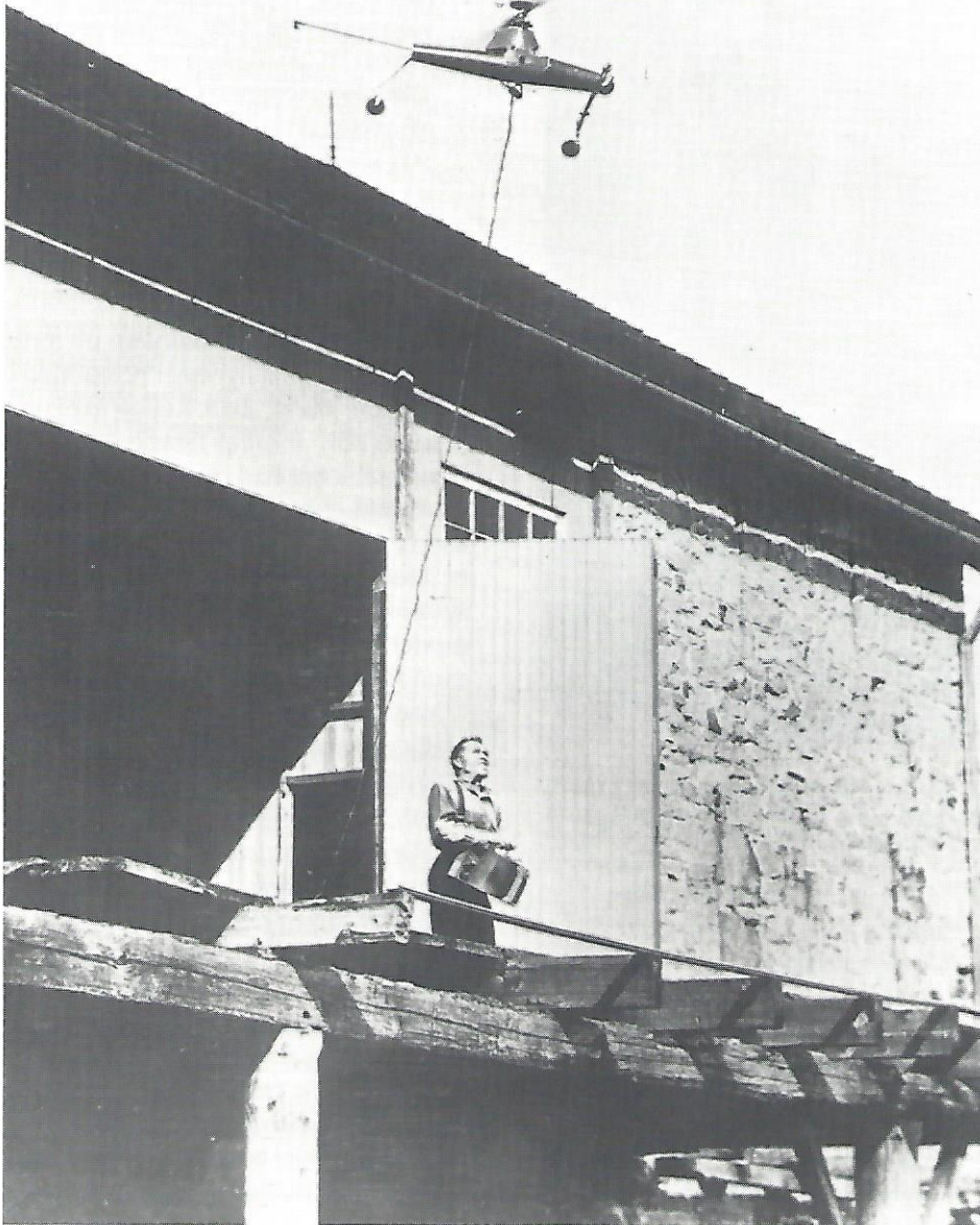
In early 1941, Young operates the famous remote control model outside his barn door. Remote capabilities were made possible by replacing the stabilizer bar with a flywheel. When time came to build a full-sized machine, the flywheel proved impractical and cumbersome. Young then reverted to the original stabilizer bar, but added mixing levers to it so that both the bar and pilot could directly control the rotor.
