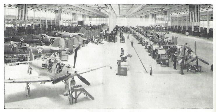
From here they fly. The end of the production line at the Niagara Falls plant. Note cleanness of line, absence of jigs and fixtures.
