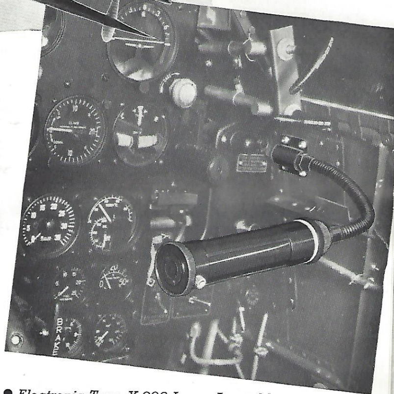
● Electronic Type X-206 Lamp Assembly installed in cockpit of Bell Airacobra.
