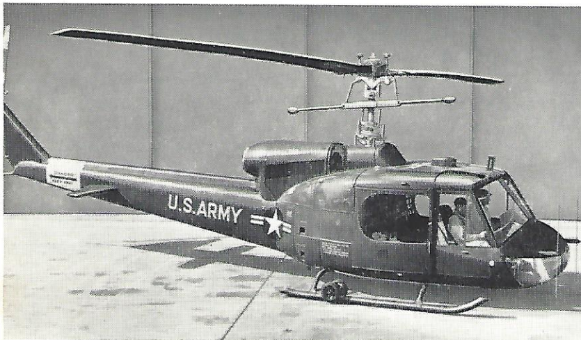
XH-40 Powered with Lycoming XT-53 shaft turbine engine, this Army utility helicopter can match climbing performance of World War II fighters.
