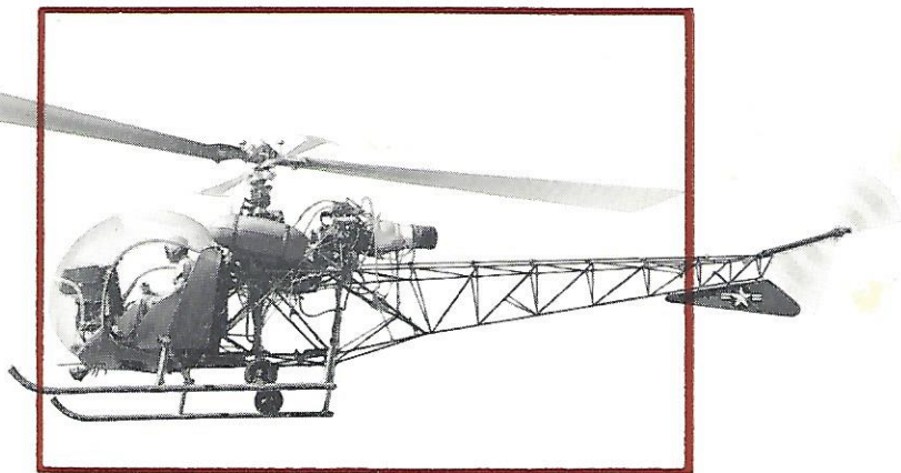
Company pilots have successfully test flown the turbo-jet powered Bell XH-13F helicopter under development for the U.S. Air Force.
