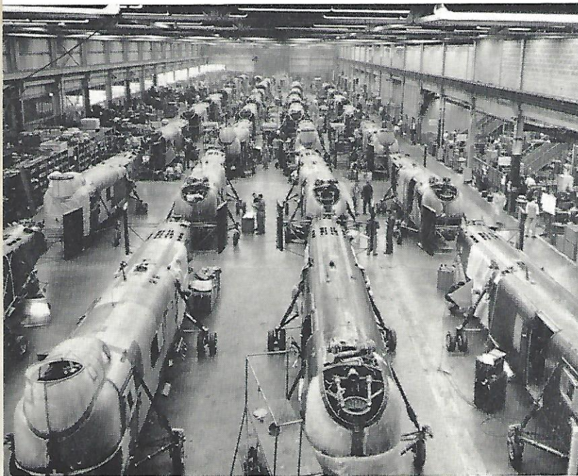
Four assembly lines of the company's big HSL-1 helicopter are in full production at the new helicopter plant in Hurst, Texas.
