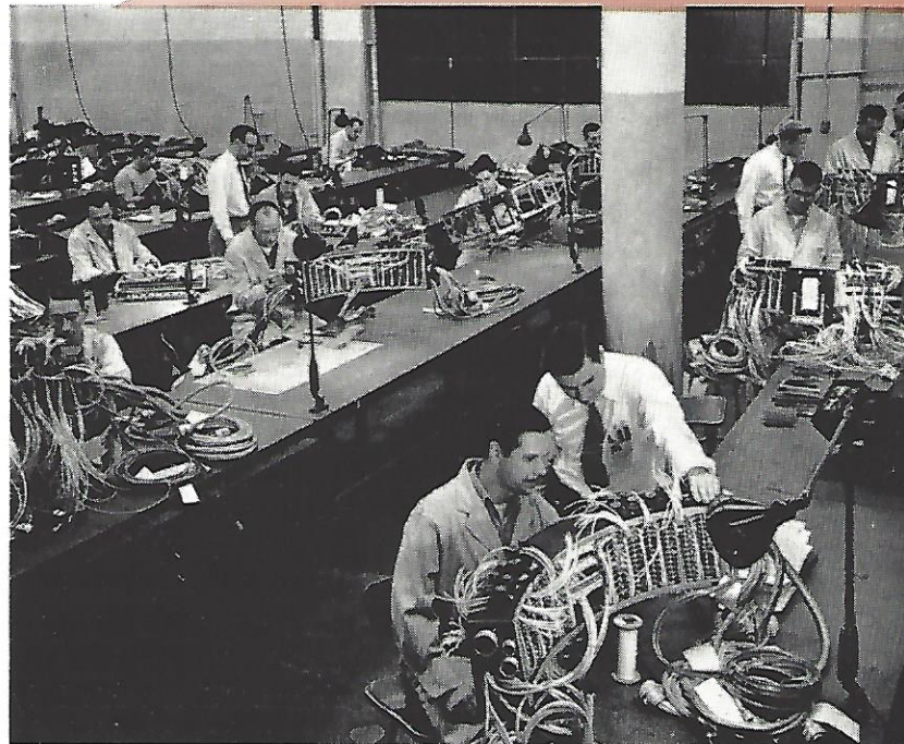
Decoders, transmitters, indicators, amplifiers and other high precision electronics and servo devices are turned out on an assembly-line basis for company's products as well as for products of other manufacturers.
