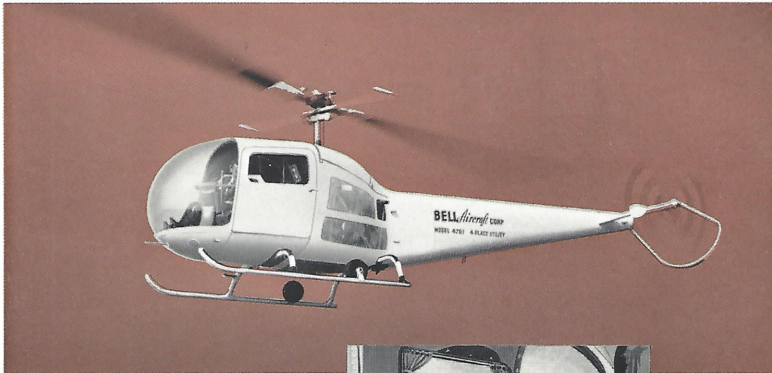
The Model 47J is the second new helicopter to be introduced in a year. It is a four-place, 250 h.p. helicopter offering five different cabin arrangements.
